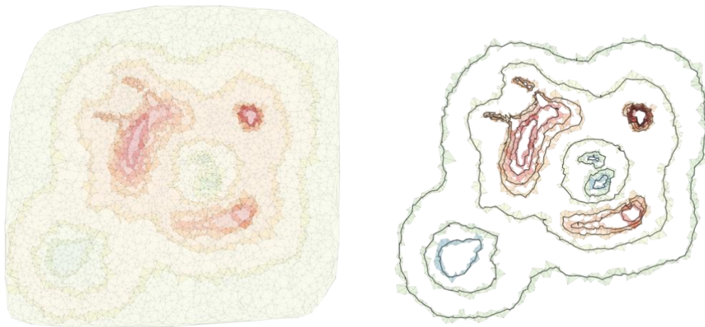
Figure 1. Geometry and generation of the TRG. (Inter-contour) regions are resembled as nodes, overlapping regions form edges. An isobath always follows such a set of edge triangles . First, triangle regions in between two isobath values are formed (b, c). If regions intersect (d), they are adjacent with each other through an edge (f). Isobaths only exist on edges, which point to the edge triangles (e).
